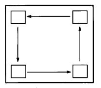
**PIP Channel Buttons** – Press the PIP CHANNEL UP or DOWN button while the PIP frame is displayed to sequentially scan through Channels.
